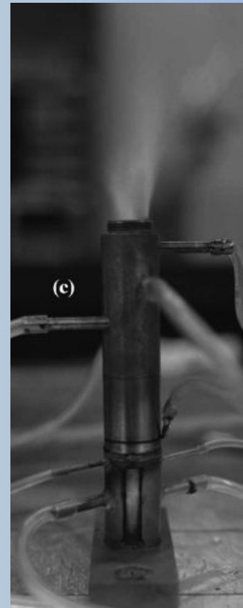
When fuel pool is present, flame condition oscillates between internal and external burning
