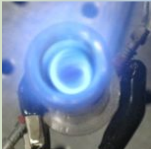
Tubular flame top view
