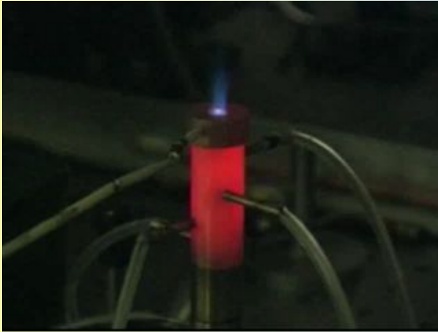
Typical swirl flow of a tubular flame
