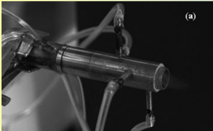
Typical swirl flow of a tubular flame
